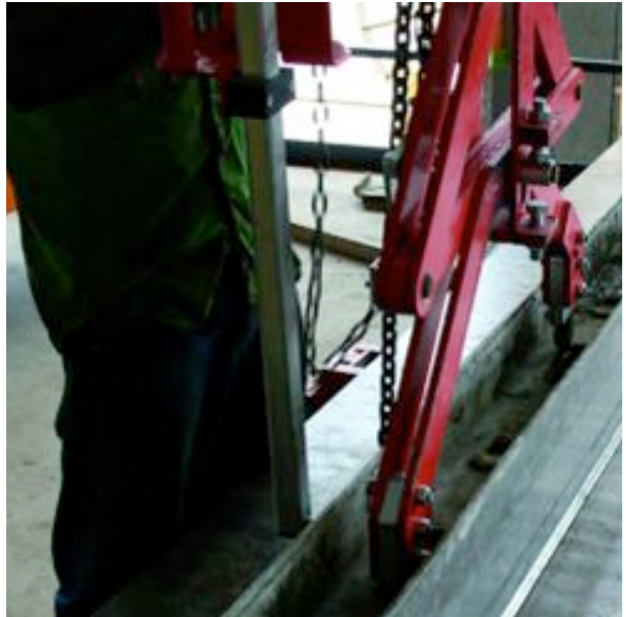
Fig. 13: A special lifting equipment enables the worker to position also heavy moulds easily
