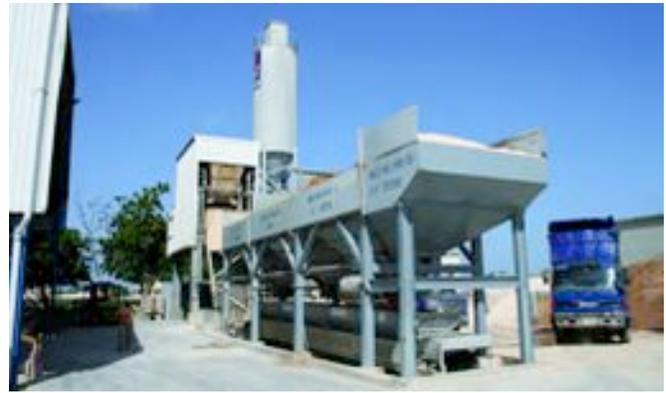
Fig. 15: The mixing plant from Elematic is serving both the dry cast and the wet cast operation
