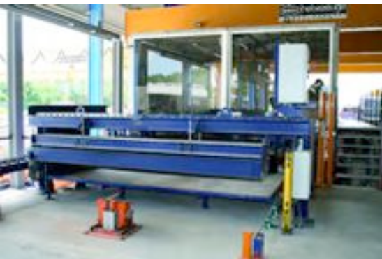
Fig. 11: A cleaning station with brushes is cleaning the pallets
