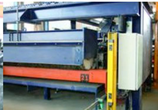
Fig. 11: A cleaning station with brushes is cleaning the pallets
