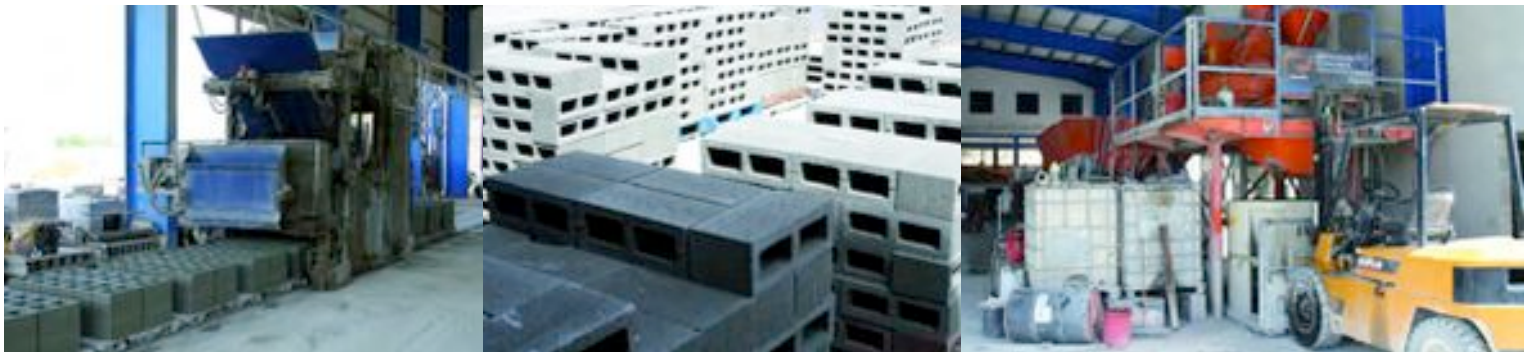
Fig. 2: A Zenith 940 multilayer concrete block machine is producing either 25,000 pavers or 10,000 concrete blocks per 8-hour shift, served by an ACT SmartMix mixing plant
