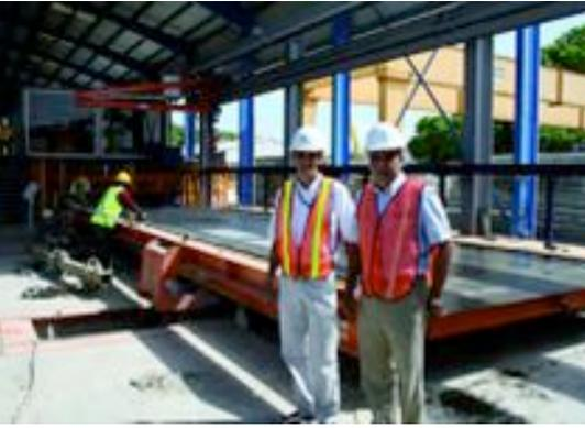
Fig. 10: The tilting station U1 is designed to enable other pallets to bypass this station during the demoulding process. Mark Maloney MD Preconco (left) and Mathias Reymann, President Ratec, are convinced that the circulation process for precast production is an optimal solution for a production of modern precast concrete walls.
