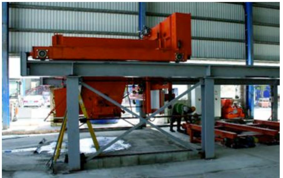
Fig. 8: The concrete distributor is served by a forklift currently. Later a flying bucket conveyor system will speed up the delivery of the concrete.
