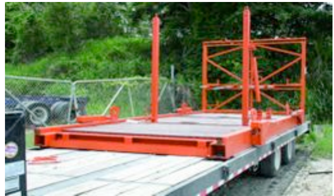
Fig. 16: Special delivery racks are used for transporting the wall panels
