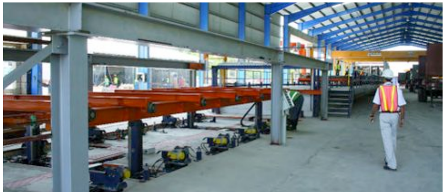
Fig. 6: A vertical circulation production plant was the solution Ratec designed for Preconco
