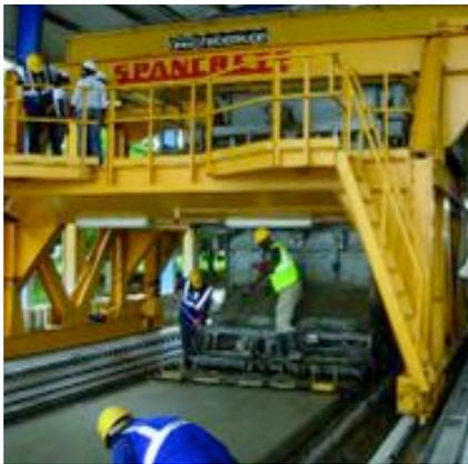
Fig 4: The Spancrete GT 240 slipformer is producing 150,000m<sup>3</sup> hollowcore slabs per year on two beds 115m long
